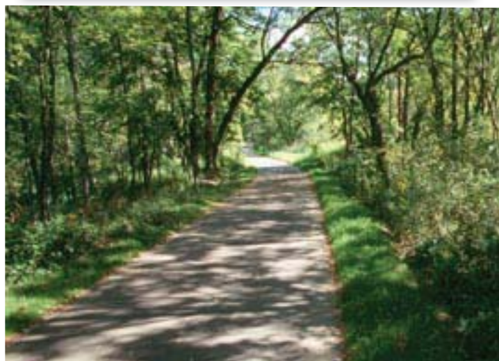
Greenway paths should be minimum 10' wide to accommodate both Pedestrians and Bicyclists
