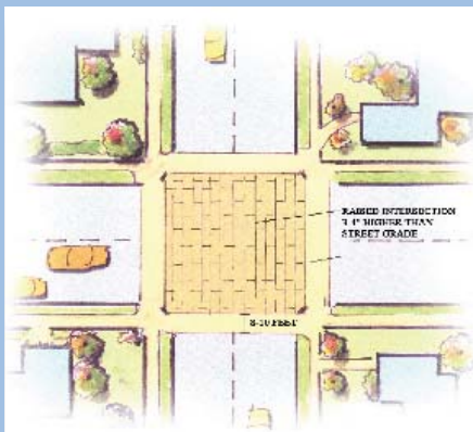
Raised intersection with decorative pavement.
