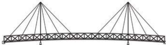
Cable-Stayed Pedestrian Truss
