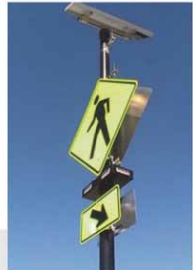
An RRFB crossing device
