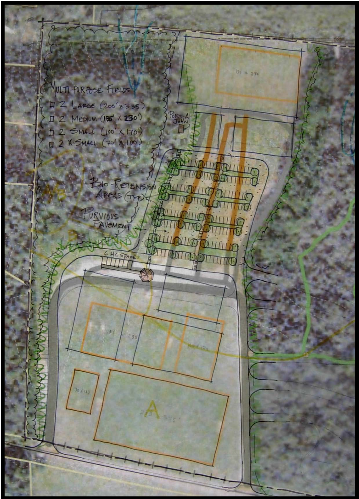
Proposed Multi-Purpose Sports Field & Pervious Parking Layout
