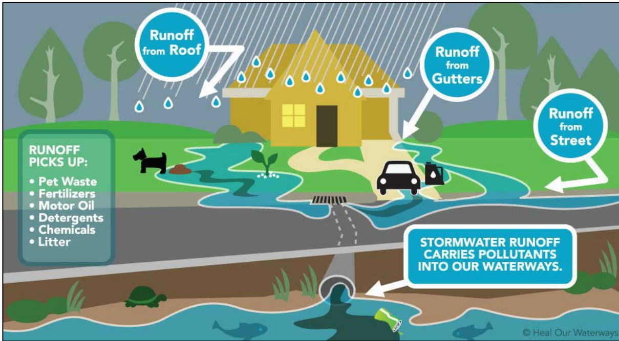
Figure 29: How Stormwater Runoff Transports Pollutants
